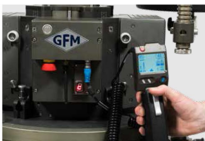
With cable connected HCU
