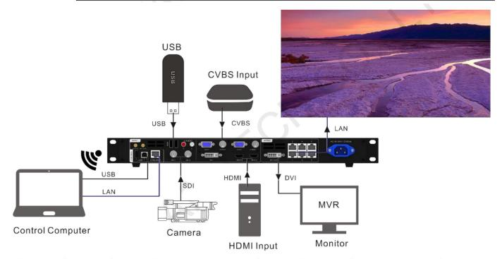
The VX5s is an all-in-one video controller, designed with powerful video processing capability that integrates sending card functions with video processing..
