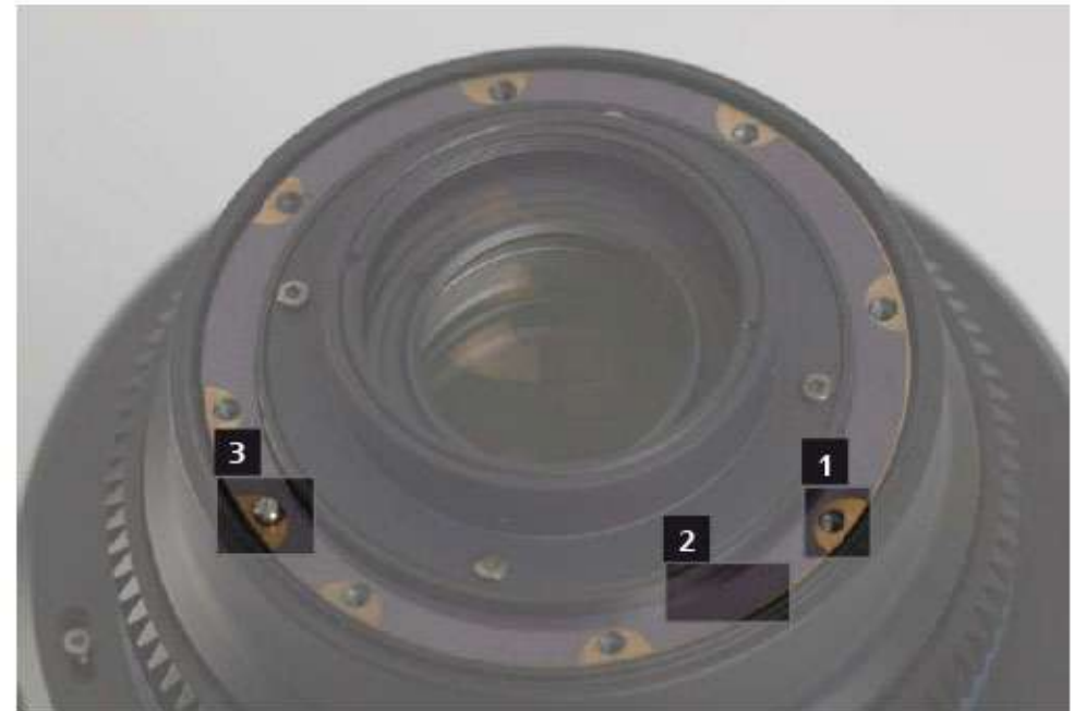
1 groove of the lens 2 shims 3 small screw in the groove of the lens
